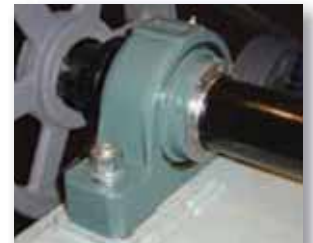
Shown with bolt on pedestal and quad split housing (option)
