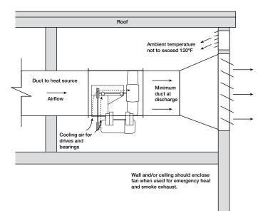
For the greatest amount of internal cooling, discharge static pressure should be kept to a minimum while keeping most of the pressure on the inlet side. Locate the fan at ends of the duct runs and near the discharge point in the system. This set-up will promote the ambient air cooling effect.
