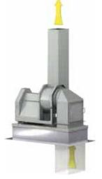
Positions the exhaust fan over the roof penetration. Compact installation minimizes roof deck space and leakage from multiple roof penetrations. Duct support provided to install duct drops in roof curb. Optional backdraft damper prevents airflow back into the building when fan is not in operation.
