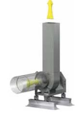
Typically used with remote fan mounting locations and ducting run along the roof deck. Slip fit or flanged connection to fan inlet. Recommended installation with three wheel diameters of straight duct prior to inlet to prevent airflow system effects.
