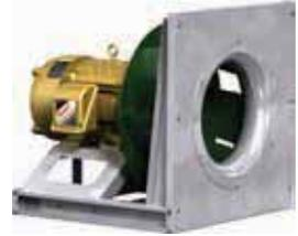
**APF** plenum fans are the ideal solution for horizontal wall mounting applications that require speed control. The Vari-Green® electronically commutated (EC) motors have integrated controls that only need a 0-10V signal (4-20 mA option), no VFD and no additional wiring required to adjust speeds. APF plenum fans are low maintenance, lightweight and have a shorter, more compact length, making it an excellent choice in multiple fan array applications or as a retrofit option.
